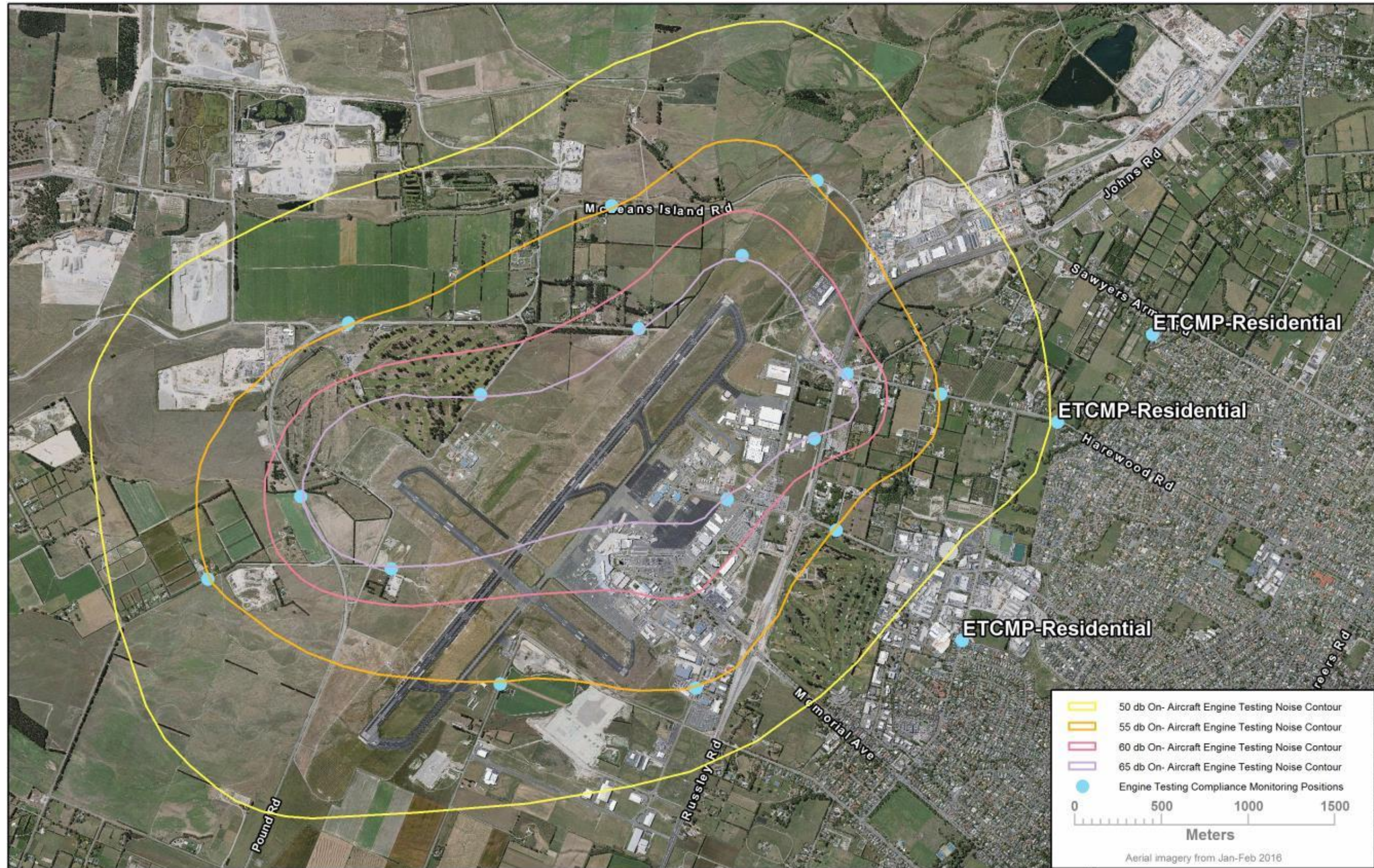
Figure 2: On- aircraft Engine Testing Compliance Monitoring Positions (ETMPs)
